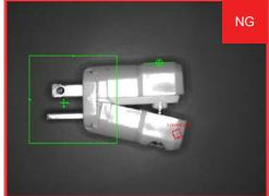
The distance between the two halves of an enclosure is measured to verify that the electrical plug has been assembled correctly. An open plug will cause a failure in the downstream packaging equipment.
