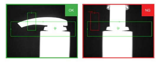
A lotion bottle is checked to confirm that the pump dispenser is in the locked position before the bottle is packed into a carton.
