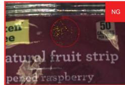
A color pixel count tool verifies that the correct fruit snack flavor is present to ensure that it is packaged in the correct order.
