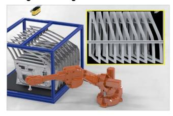
Vision-guided robotics helps move stamped parts from the line to a rack for inspection and identification.
