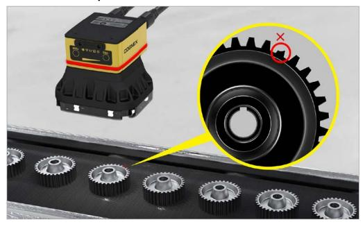
Machine vision systems gauge the dimensions of transmission gears and inspect for damage.
