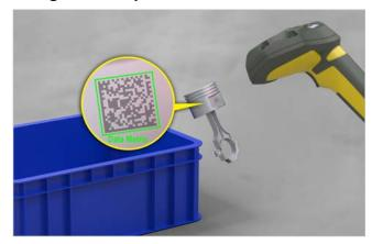
Barcode readers verify that a kit contains the correct parts so vehicles spend less time at each assembly station. This results in more vehicles produced each day.
