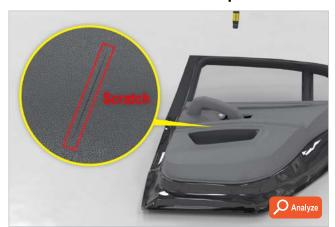
Deep learning, diffused direct light, and HDR+ image formation technology helps separate and identify defects from the normal surface area of the inside door material.
