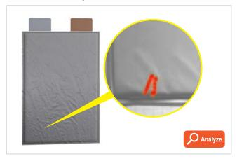
Cognex deep learning vision software identifies surface defects, like bubbles and wrinkles, on a pouch's surface.
