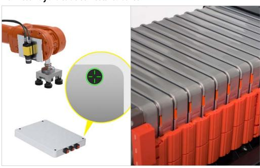
Machine vision systems guide the final assembly of modules and cable connectors into a pack.
