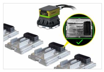
Vision systems identify transmission module components prior to assembly.
