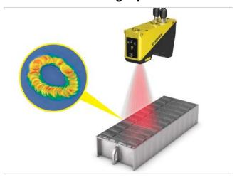
3D laser displacement sensors and Cognex deep learning vision software inspect the welds on a battery pack's modules and busbars.
