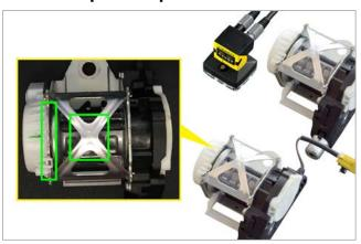
Vision sensors confirm the presence of critical features and dimensions of seatbelt components prior to assembly.
