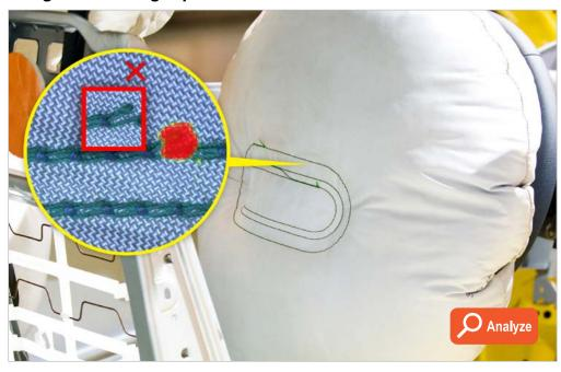
Deep learning vision software inspects the stitching on airbag fabric and stitching for defects.
