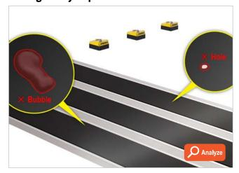
Cognex industrial line scan cameras and Cognex ViDi deep learning vision software detect defects such as craters, bubbles, and holes on electrode sheets.
