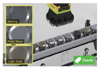
Deep learning vision technology inspects the presence of the proper FPA by color as well as the FPA seal presence and proper insertion.
