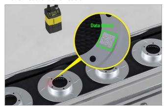
Barcode readers identify components for the brake assembly, even on highly reflective surfaces.
