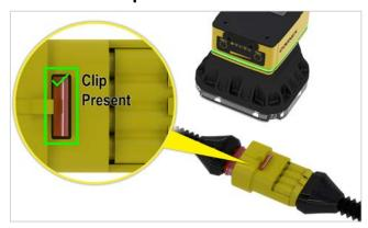
Detect the proper insertion of the seat connector by detecting the red clip presence via PatMax.
