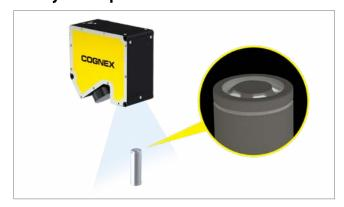
3D laser displacement sensors inspect the dimensions of battery caps to ensure they are fully sealed and free of defects. They use a highly accurate telecentric lens to accurately capture grooves and any defects like tilting or uneven height, regardless of the can's color.
