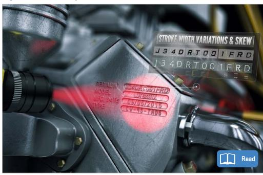
Vision systems with optical character recognition (OCR) read codes to track and trace engine blocks.
