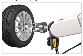
Machine vision systems guide robotic arms to help locate and properly torque a wheel's lug nuts.
