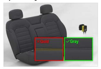
Detect and verify the correct color of vinyl and stitching for interior components such as seats, headrests, and doors.
