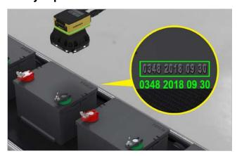
Machine vision systems verify the presence and placement of battery terminals and identify them by their alphanumeric codes.
