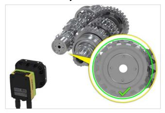
Vision systems inspect that the transmission has been assembled correctly.
