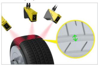
3D laser displacement sensors verify treads' critical dimensions.
