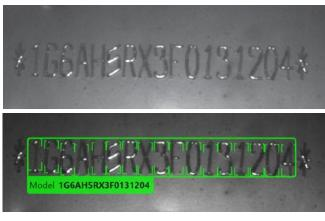
Deep learning vision software reads the deformed characters marked on a VIN code for traceability.
