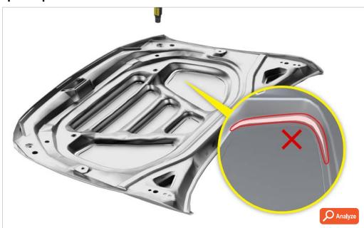
Detect the presence and gauge the width of an opening within a stamped piece of metal.
