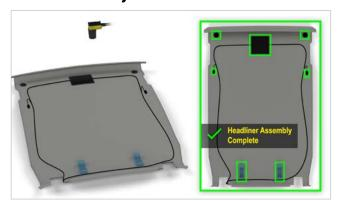
Machine vision systems detect the presence and absence of headliner components and verify the part has been assembled correctly.
