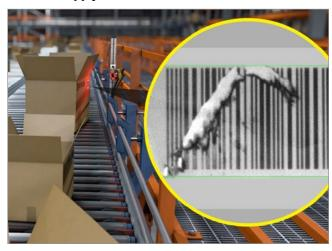
Image-based barcode readers catch label print and placement issues early on, allowing facility managers to identify and fix label or printer errors to minimize problems downstream.
