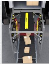
Overhead presentation reading stations or multi-reader barcode scan tunnels decipher codes on various sides of a package, at extreme angles, and different orientations reducing rework and lowering costs.
