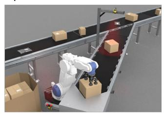
Image-based barcode readers use advanced algorithms and decoding technology to quickly read codes on parcels and packages entering the sorting system, adding traceability and efficiency to the sorting process.
