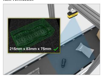
The 3D-A1000 Dimensioning System quickly and accurately captures volume and dimensioning data of picked items which increases order accuracy, improves inventory management, and lowers return costs.
