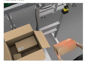
Cognex image-based barcode technology quickly reads omnidirectional, damaged, smudged, and distorted codes and codes at extreme angles, improving pick and pack sorting times and maximizing throughput.
