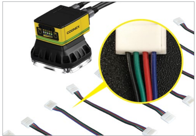
Machine vision systems inspect electrical modules for color and quality prior to assembly.
