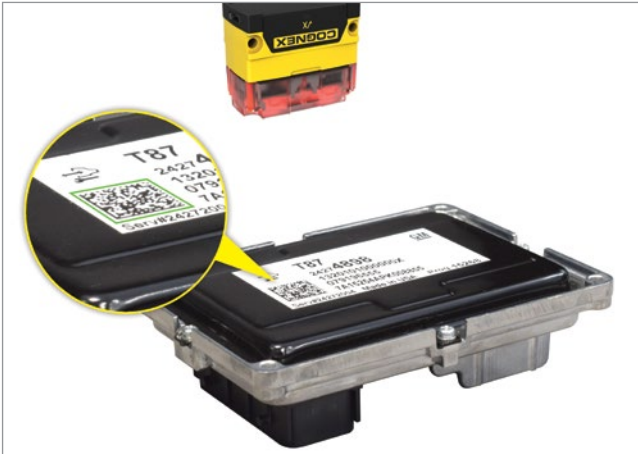
Barcode readers identify and sort electrical components.
