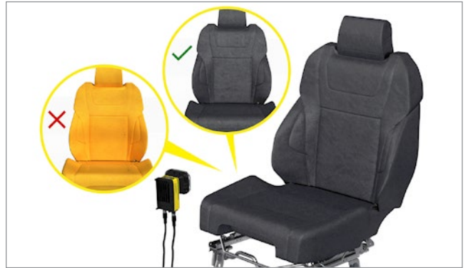
Cognex Deep Learning confirms that the right covers have been correctly installed on automotive seats.
