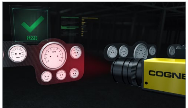
A machine vision system verifies the presence, proper spacing, alignment, and completeness of a dashboard.
