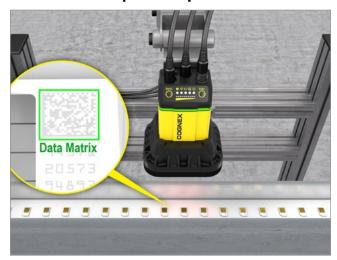
DataMan fixed-mount barcode readers easily and reliably read 2D codes on small components thanks to fast read rates and powerful decoding algorithms such as PowerGrid technology.
