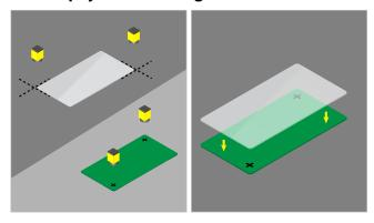
AlignPlus software aligns display components relative to each other using unified multi-camera motion stages.
