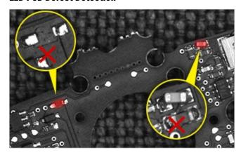
Cognex Deep Learning can reliably learn and detect various anomalies of LEDs and other components on PCBs which improves overall board quality.
