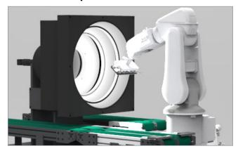
Available in Asia only, Cognex's Cosmetic Optical Inspection (COI) system identifies and classifies defects simultaneously on multiple surfaces under ideal lighting conditions.
