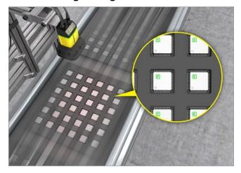
Cognex DataMan image-based barcode readers reliably read 2D codes on integrated circuits enabling traceability.
