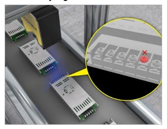
3D laser displacement sensors determines with high precision whether the height of the screw is outside the accepted range.
