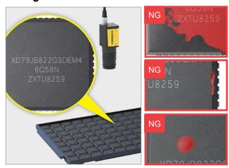
Cognex Deep Learning technology identifies and classifies a wide variety of functional defects, such as cracks or voids on IC molding to help increase IC quality.
