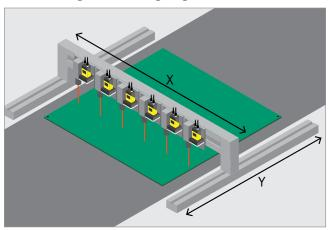
AlignSight sensors perform vision-to-motion control calibration quickly and automatically to ensure precise alignment between the drill and PCB boards.
