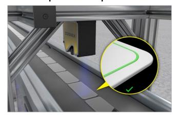
3D laser displacement sensors assess glue adhesion volume dimensions and position on the part.
