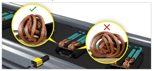
Cognex Deep Learning's defect detection tool easily finds unacceptable functional defects on complex braided wire connections so only acceptable connections are passed forward in the process.
