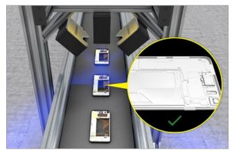
2D and 3D vision systems verify that components are properly installed and meet quality parameters.
