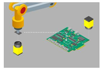
Machine vision solutions guide components, including surface mount devices, onto PCBs.
