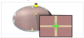
PatMax technology provides robust, accurate, and fast wafer and die pattern location for wafer inspection, probing, mounting, dicing, and testing equipment.
