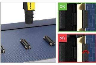
Cognex Deep Learning's defect detection tool identifies both cosmetic defects and functional defects on BTB connectors that cause quality issues.
