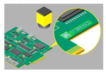
Barcode reading technology identifies serial numbers on board components and reads codes on PCBs for traceability.
