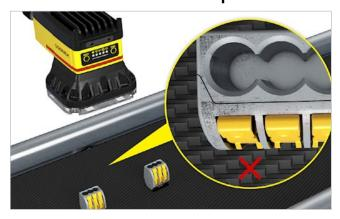
Cognex Deep Learning detects anomalies anywhere on the electrical connector ensuring only acceptable connectors move forward in the assembly process.
