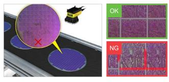
Cognex Deep Learning defect detection tool learns the difference between acceptable and non-acceptable defects on wafer surfaces.
