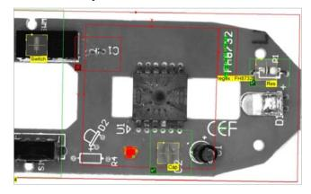
Cognex Deep Learning quickly and reliably solves mouse PCB assembly verification by learning the difference between good and bad PCBs.
