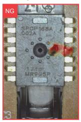
Cognex Deep Learning learns the normal appearance and position of a chip's leads and pins and characterizes all features that deviate as defective.
