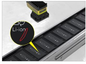
Cognex Deep Learning checks the integrity of batteries and differentiates between cosmetic and functional anomalies.
