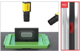
Cognex Deep Learning learns the variable defects like rips, weak spots and missing glue marks associated with LIM rubber seals used in smartphones.
