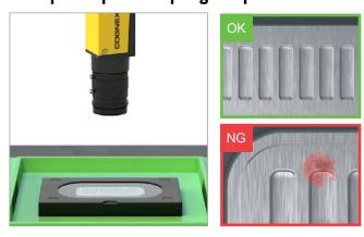
Cognex Deep Learning defect detection tool learns the difference among the wide range of cosmetic and functional adhesion anomalies on smartphone speaker diaphragms.
