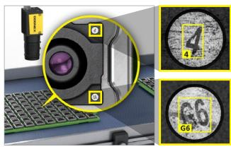
Cognex Deep Learning's OCR capability accurately reads damaged alphanumeric codes used to orient camera lenses of various diameters into multi-size lens holders.
