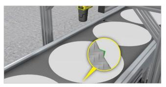
In-Sight vision systems and PatMax accurately identify the wafer's notch and XY position in any orientation.
