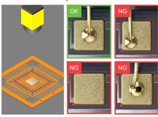
Cognex Deep Learning defect detection tool learns and correctly identifies the wide variety of wire bond welding defects which can affect IC performance.
