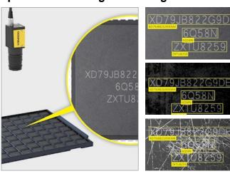
Cognex Deep Learning's OCR capability improves traceability by accurately reading damaged alphanumeric codes in ICs, even on difficult backgrounds.
