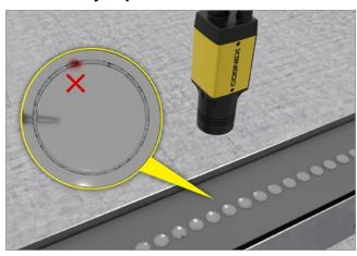
Cognex Deep Learning's defect detection tool finds functional defects while minimizing false positive from purely cosmetic defects.
