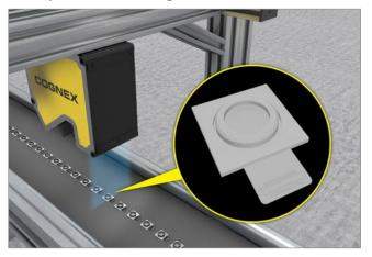
3D laser displacement sensor gauges the height dimensions for a complex, transparent camera assembly.
