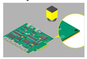
PatMax uses geometric information to locate fiducial marks during screen printing, glue dispensing, mounting, and automated optical inspection.
