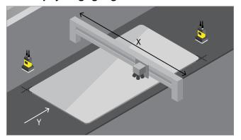
AlignSight sensors and PatMax vision tools locates trained patterns so the gauging robot begins their job on the same location of the OLED display every time.
