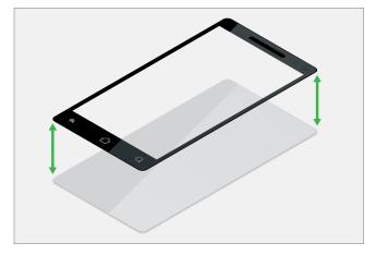
AlignPlus software quickly and with high precision automatically aligns the glass to the stencil.
