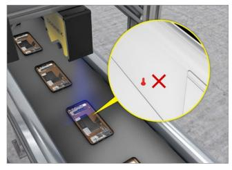
3D systems ensure the module mounting area is free of potential obstructions.
