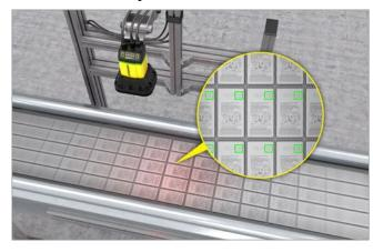
DataMan barcode readers decipher multiple direct part mark codes on high-speed production lines.
