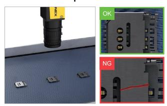
Cognex Deep Learning's defect detection tool learns the difference between cosmetic and functional defects on SIM card connectors.
