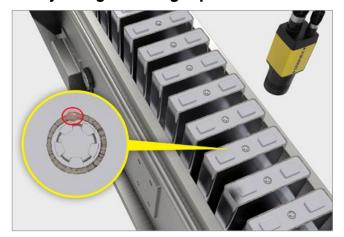
Cognex Deep Learning combined with a 3D laser displacement sensor inspects for weld defects and that the sealing pin is placed correctly.
