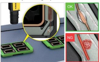
Cognex Deep Learning checks the integrity of batteries and Cognex Deep Learning searches for and detects a wide variety of functional defects of smartphone voice coil spot welds.
