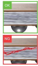
Cognex Deep Learning learns the normal appearance of the sidewall of a WLCSP and characterizes all features that deviate as defective.
