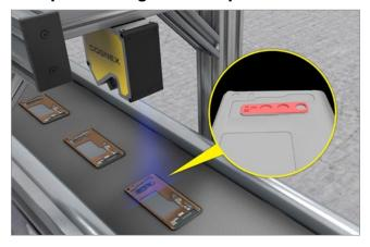
3D laser displacement sensors gauge the height and detect the smallest dents to micron-level accuracy.
