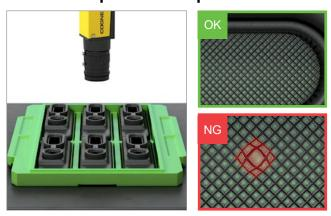
Cognex Deep Learning's defect detection tool identifies contamination or cosmetic defects anywhere on the part.
