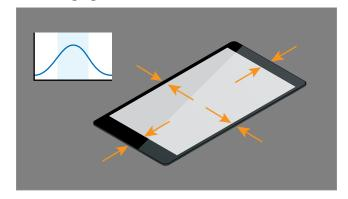
In-Sight systems and AlignPlus software gauge the alignment accuracy of parts based on specific features that do not have to be in the camera's field of view.
