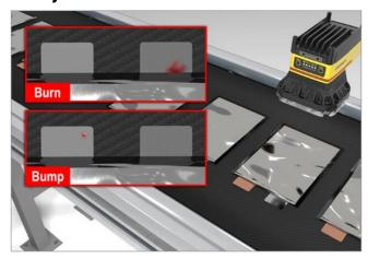
Cognex Deep Learning's defect detection tool flags any battery tabs or solders that are outside the acceptable range.
