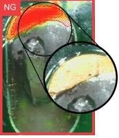
Cognex Deep Learning locates solder resist on a diode despite specular glare and identifies a wide variety of defects such as bridging, peaking, and gapping.
