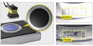
Cognex Deep Learning's OCR capability improves traceability by accurately reading worn and damaged alphanumeric codes on wafer carrier rings.
