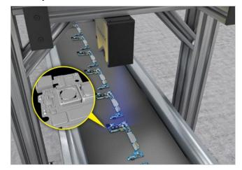
2D and 3D machine vision systems inspect PCBs for the proper number, size, and placement of components.
