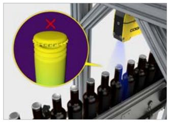
Ensure the bottle is properly sealed by checking the height and tilt angle of the bottle cap.
