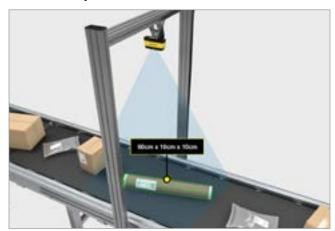
Collect dimensional and volumetric information for outgoing freight, enabling outbound handlers to pack their trucks efficiently to optimize transportation costs.
