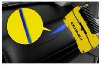
Ensure proper alignment of airbag compartment cover and flushness with the dashboard.
