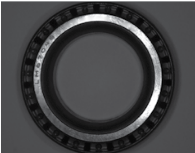
Without HDR: Embedded parts are unclear.
