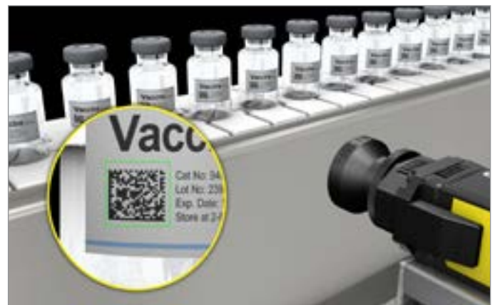
Packaging track and trace: Decode a range of barcodes for reliable, end-to-end traceability
