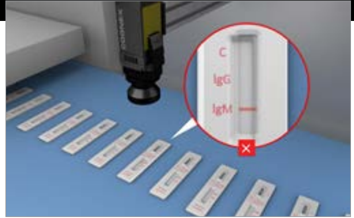
Presence/absence detection: Identify damaged or missing components to ensure product integrity
